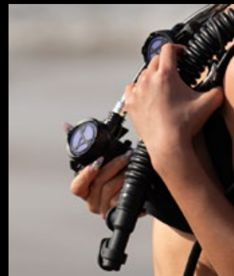
Venturi lever to prevent free flow
